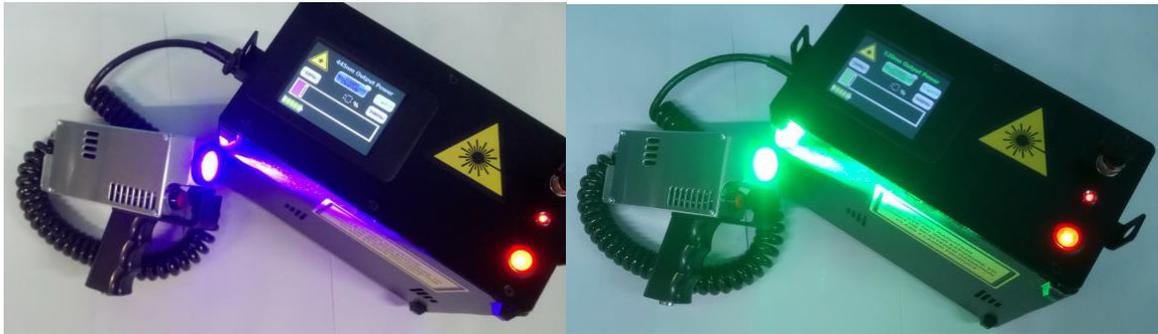
The **Revelation 445/532 nm Dual wavelength forensic** from Laser Innovations Ltd is a widely used a validated laser system for evidence recovery. The lightweight design (4 kg) provides 2 laser guns one Blue and one Green which are both easy to clean with 10% bleach solution. This laser provides 10 Watts Blue at 445nm and 8 Watts Green at 532nm.
